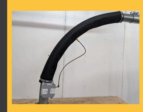
Install the remaining end gasket sliding inside the sleeve.
